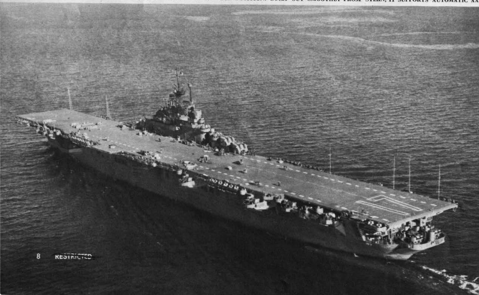
STERN CLOSE-UP OF U.S.S. BUNKER HILL SHOWS "BUSTLE" GUN POSITION. BUILT OUT SMOOTHLY FROM STERN, IT SUPPORTS AUTOMATIC AA
